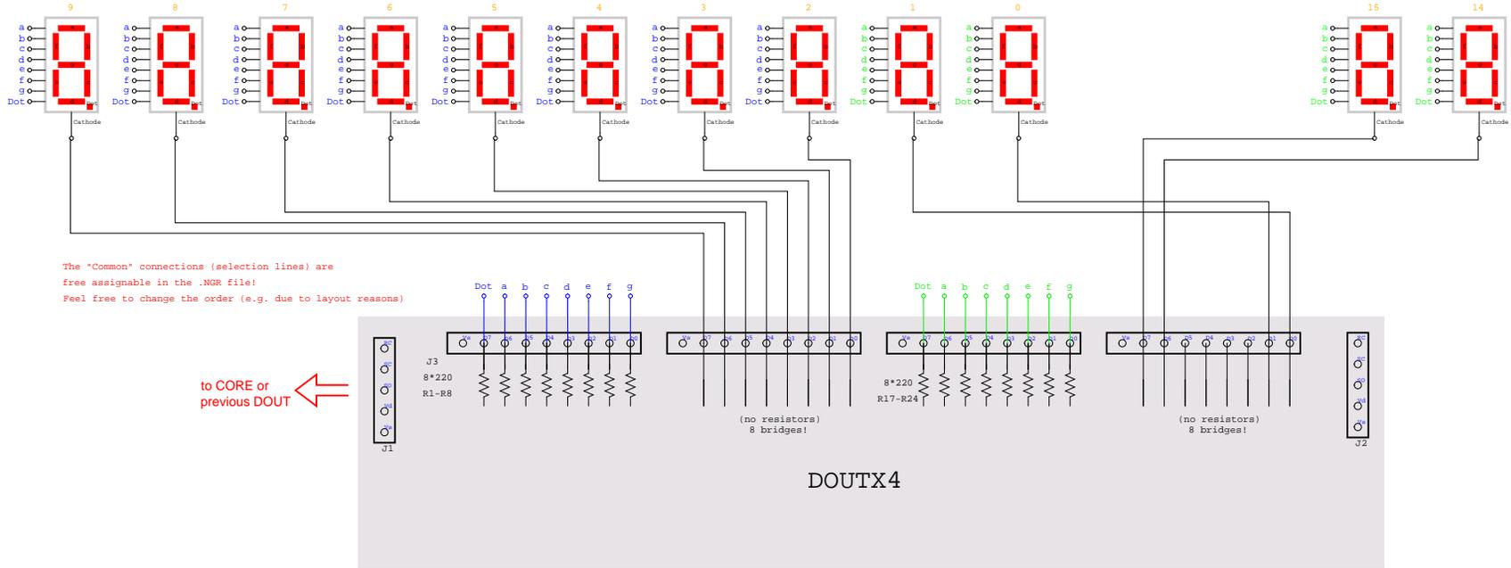
The \*Common\* connections (selection lines) are free assignable in the .NGR file!
